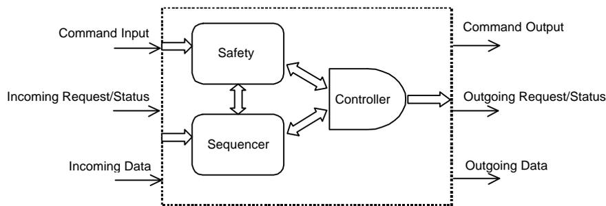
**Fig. 3.** An example of a generic subautonomy
