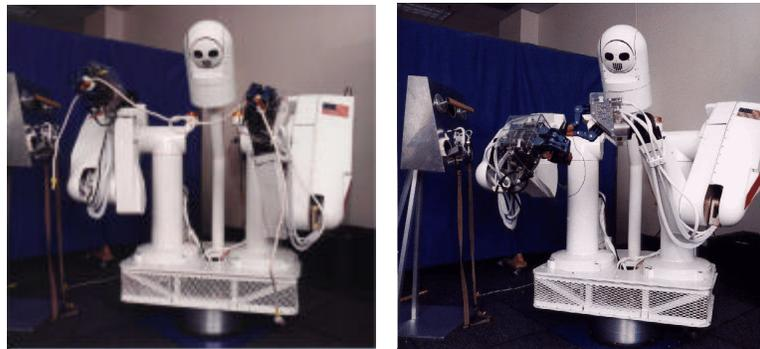
**Fig. 1.** DART tying a knot and cutting wire
