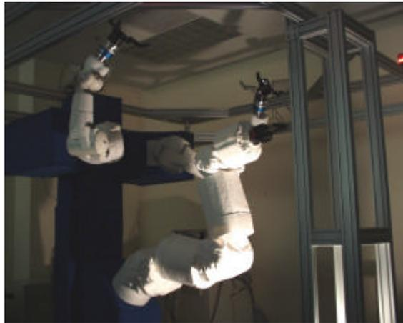
**Fig. 7.** Cooperative Manipulation Testbed (CMT)
