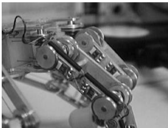
Fig. 5. Hall-Effect Based position sensors mounted on the finger of the hand
