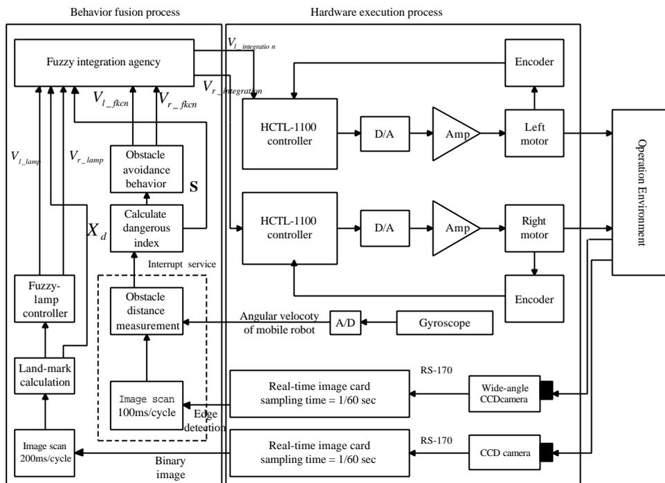
**Fig.7.** System block diagram of the navigation system
