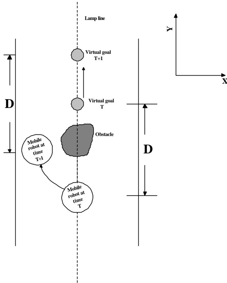
Fig.8. Setup of the virtual targets
