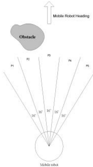
**Fig.1.** Obstacle detection using a wide-angle CCD camera
