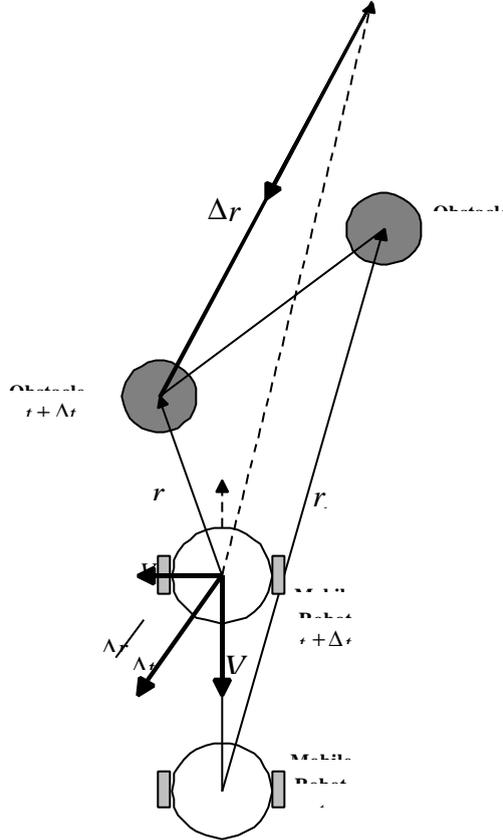
**Fig.2.** Relative velocity between an obstacle and the mobile robot
