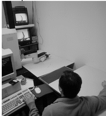
Figure 7. Anthropomorphic robot arm imitates the movements of master arm.
