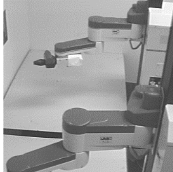
Fig. 19. Master arm and slave arm: imitation in 3D.
