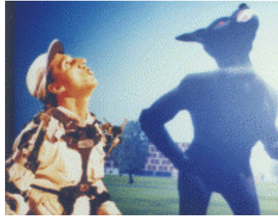
Fig. 6. Operator in Sarcos' SenSuit controls a virtual anthropomorphic creature (Copyright Sarcos Inc, reprinted with permission)
