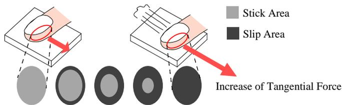
Fig. 2. Behavior of Contact Surface when Tangential Force is Applied
