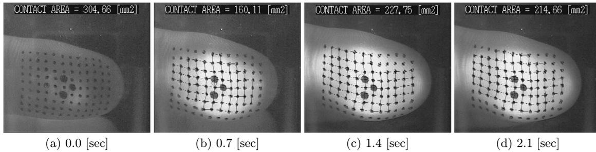
Fig. 11. Processed Image under Normal Condition
