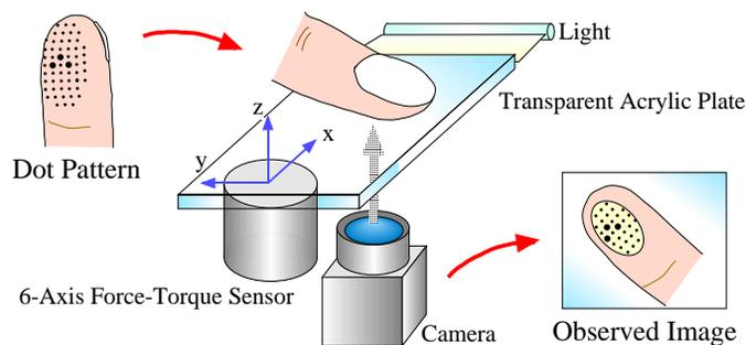
Fig. 4. Simultaneous Measurement Method of Incipient Slip and Contact Force
