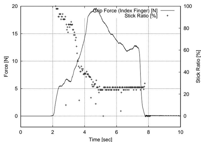
Fig. 13. Profile of Grip Force and Stick Ratio under Slippery Condition
