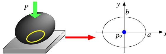
Fig. 1. Shape of Contact Area when Smooth Elastic Object Contact with Rigid Plate
