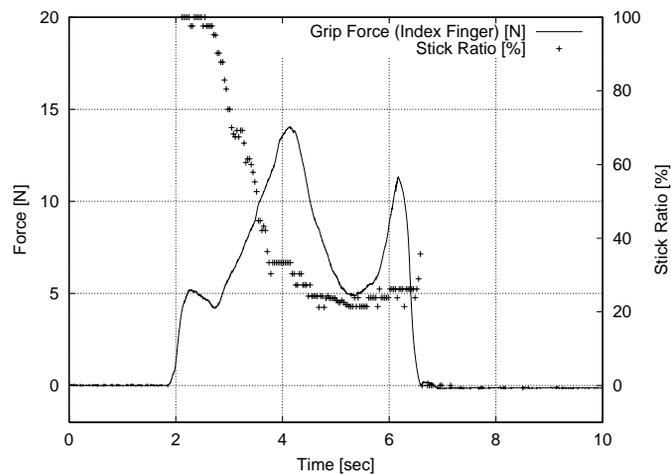
Fig. 12. Profile of Grip Force and Stick Ratio under Normal Condition
