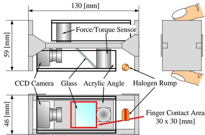
Fig. 6. Structural Figure of the Measurement Device
