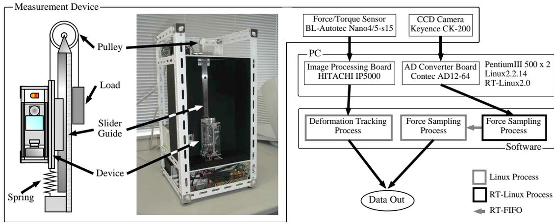
Fig. 8. Structure of the Experimental System
