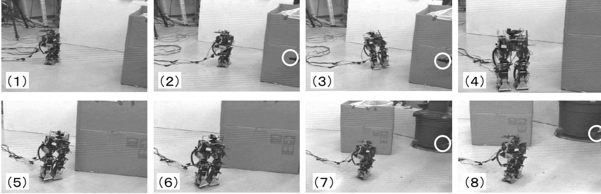
Fig. 10. The robot approaches the goal while avoiding the obstacle.
