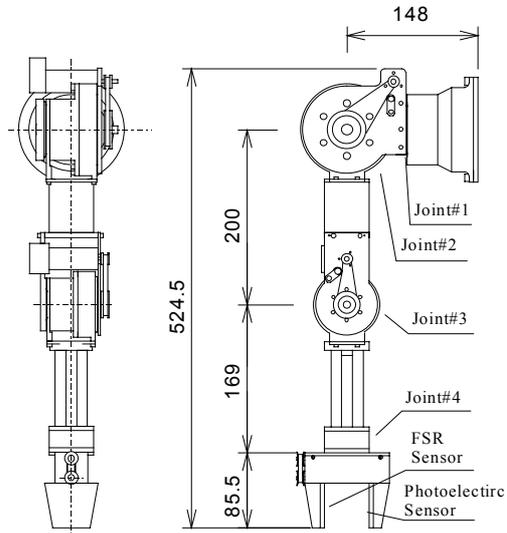
Fig. 1. Assembly draw of WAMOEBA-2R Arm-Hand Mechanism
