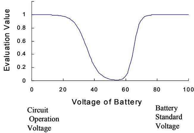
**Fig.4** Evaluation Function of Voltage Battery
