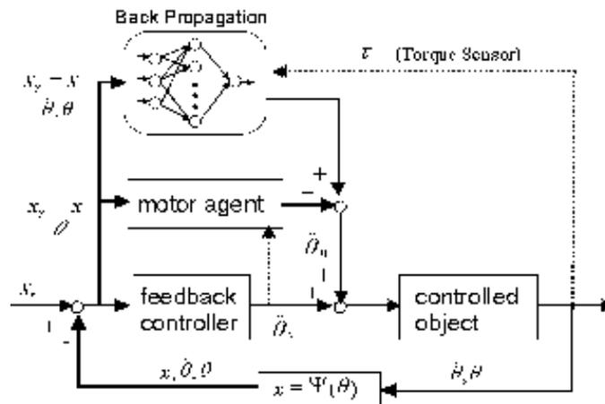
Fig. 5 Block Diagram of Wamoeba-2R Arm Control
