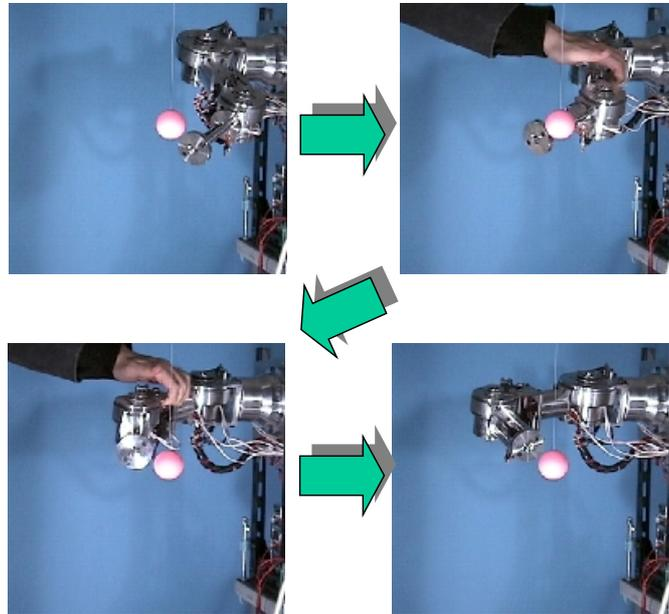
Fig. 6 Physical interaction between human and Wamoeba-2R arm
